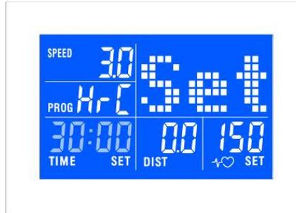
Press START: the treadmill will run at 3 km/h for 2 minutes as warm-up: adjust elevation manually.
