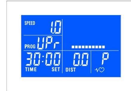
Use  $\uparrow/\downarrow$  buttons to program speed and incline for each segment, press ENTER to confirm.
